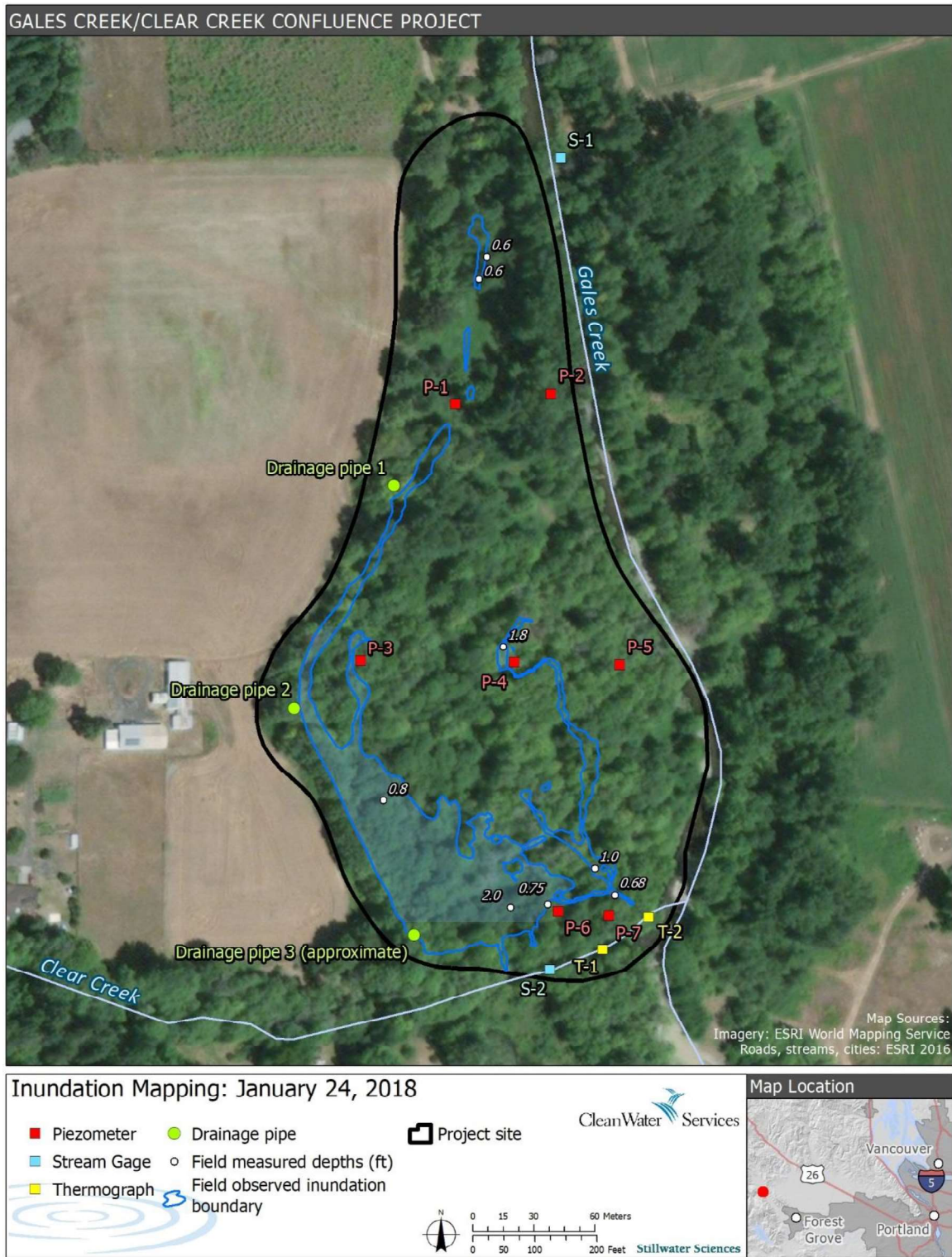
Figure 16. Map of field-based delineation of floodplain-inundation extent (polygons) and measurements of inundation depth (points) during wet-season conditions in January 2018 before enhancement construction.
